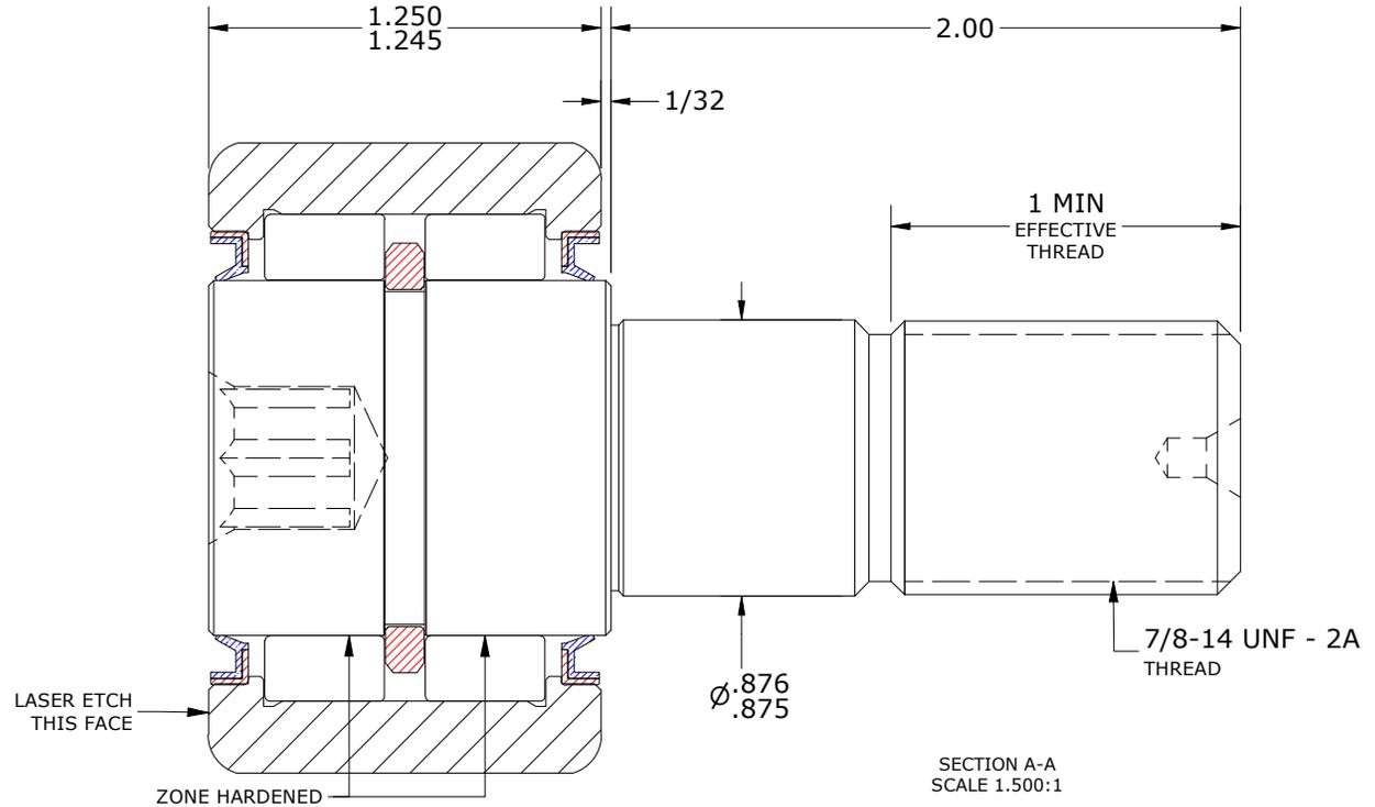
\*\*TORQUE SPECIFICATION IS BASED ON LUBRICATED THREADS, IF USING DRY THREADS DOUBLE TORQUE VALUE
