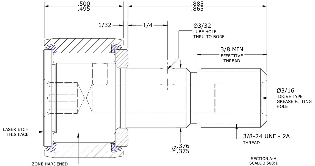
\*\*TORQUE SPECIFICATION IS BASED ON LUBRICATED THREADS, IF USING DRY THREADS DOUBLE TORQUE VALUE
