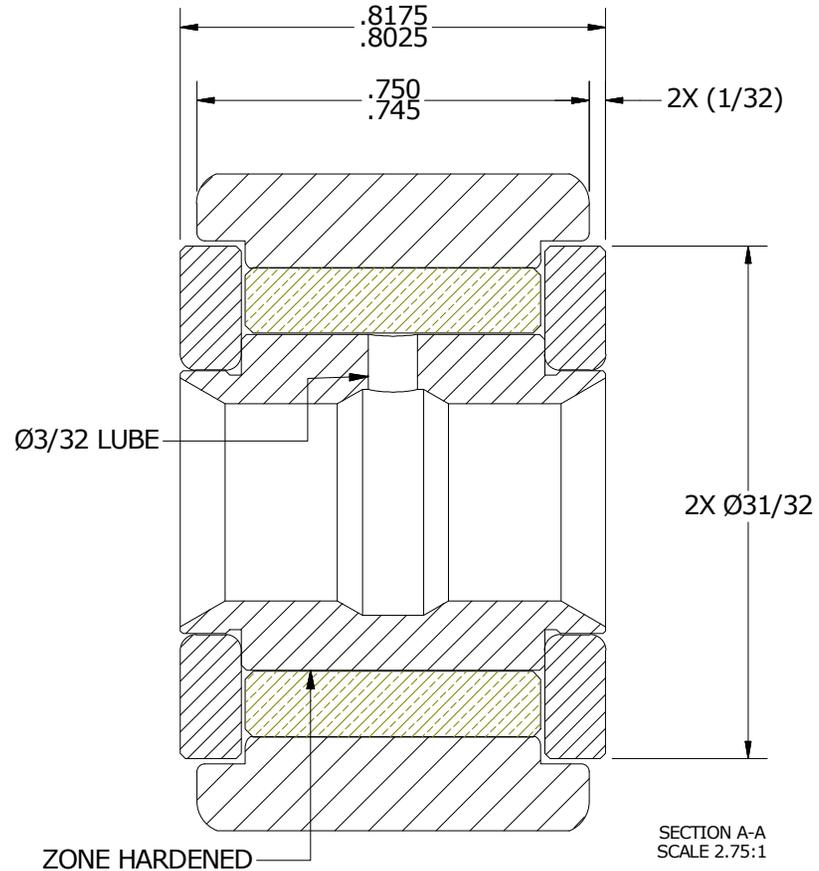
MATERIAL NOTES: OUTER RING - BEARING STEEL, HEAT TREATED
